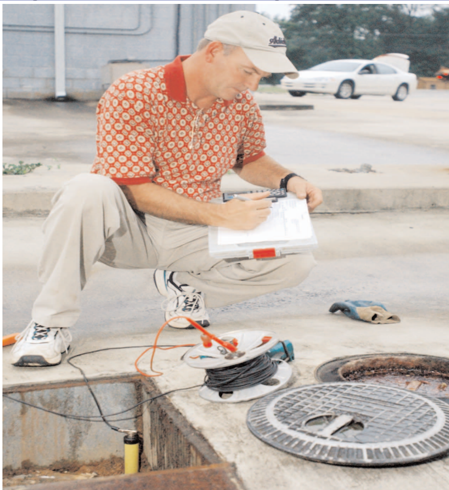
After placing a reference cell in soil near the sump box, Harry Little double checks some data. (Photo by Woody Marshall)
