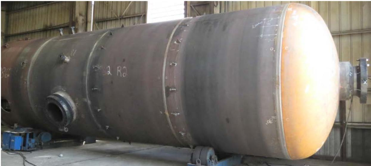
**A vertical drum made using SA-516-70.**
