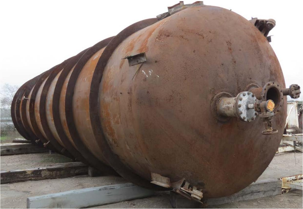
This vessel is a vacuum tower made of SA-285C from the 1950's.
