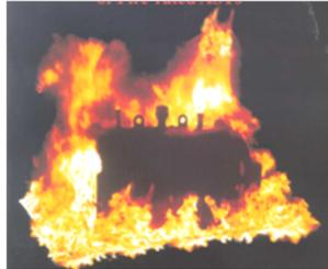
The purpose of the test was to safely assimilate an underground storage tank environment with aboveground tank installations that dispense motor vehicle fuels.
