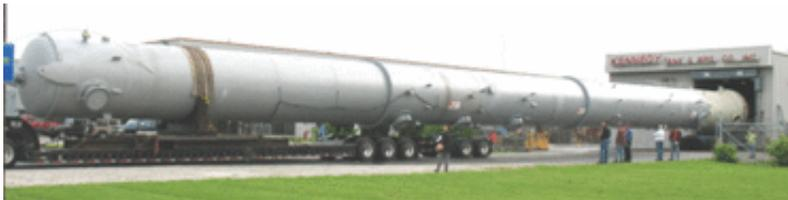
The monstrous vessel, used in a proprietary manufacturing process, weighed 250,000 pounds, was made of 1-inch thick steel, measured 9' in diameter and was 175 feet long.
