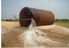
The strength of steel was proven yet again by an STI member when a UL 58 steel tank was hydro-tested to failure. The tank ruptured at 110 psi. UL 58 tanks are intended to operate at atmospheric pressure and are factory leakage tested at 5 psi.
