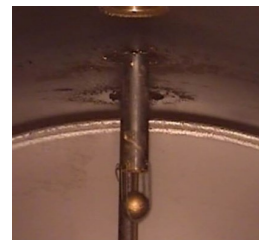
Corrosion on fittings in an FRP tank (left) and a steel tank (right). Both tanks store ULSD.
