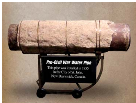
Cement mortar lined and coated steel pipe that was installed in 1855 in the City of St. John, New Brunswick, Canada.
