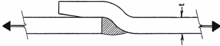
**Figure 10.** Joggle joint for pressure vessels.
