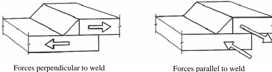
**Figure 11.** Relationship of direction of forces to the direction of fillet welds on lap-welded joints.
