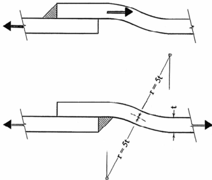
**Figure 9.** Single-welded lap joint (fillet weld) Outside weld (top) and inside weld (bottom) Double welded lap joint is both combined.
