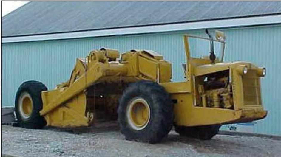
**Figure 7.** Tournapull – one of LeTourneau’s inventions – became the carryall loader.
