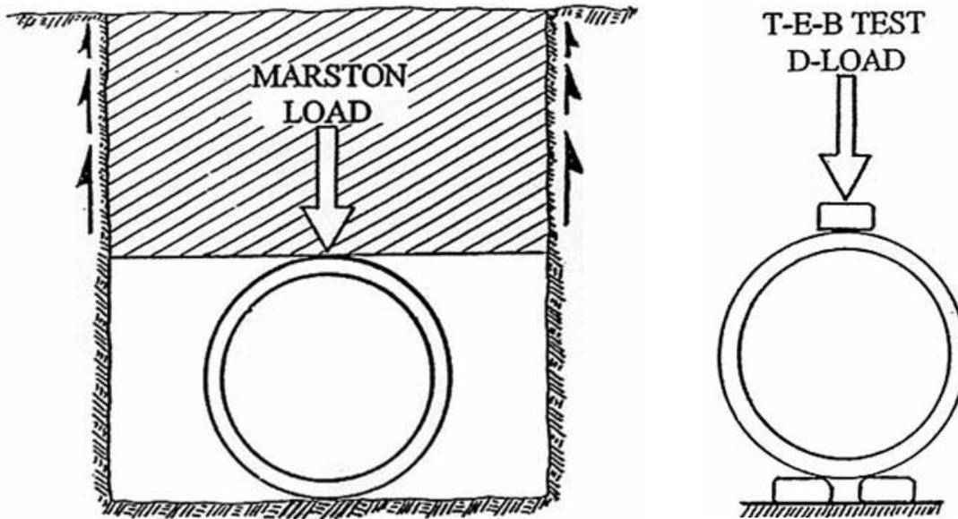
**Figure 3.** Marston load on buried concrete culverts was the weight of the backfill reduced by friction of the trench walls; and the D-load test for manufacturers to meet the Marston Load requirement.
