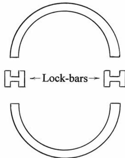
**Figure 4.** Sketch of Lock-bar pipe.
